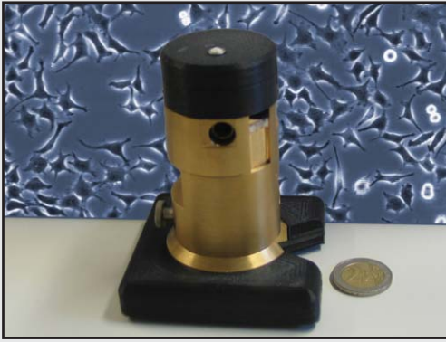
Image: No bigger than a soda can, the small-scale incubator microscope is a space-saving and cost-effective solution for time-lapse observation of cell cultures (Photo courtesy of Fraunhofer IBMT).
