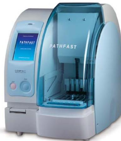
The PATHFAST is a compact, fully-automated, bench-top chemiluminescent immunoassay analyzer that provides rapid measurement of cardiac biomarkers from whole blood samples in less than 17 minutes. With the PATHFAST, physicians are able to obtain quality results quickly and accurately, enhancing patient care.
